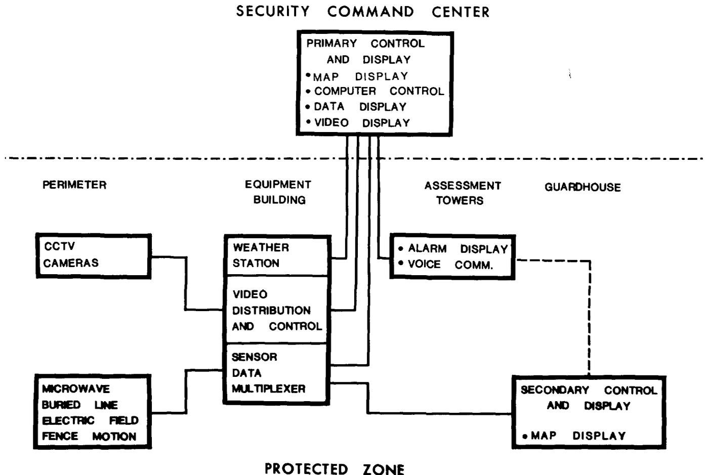
Figure 1. Simplified Security System Block Diagram
