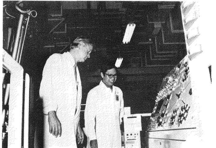
Examining the main control panel of spent-fuel-element chopping machine.
