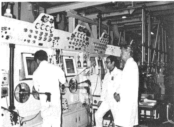
**Sample preparation by remote operation in hot cells of the analytical laboratory at Tokai.**
