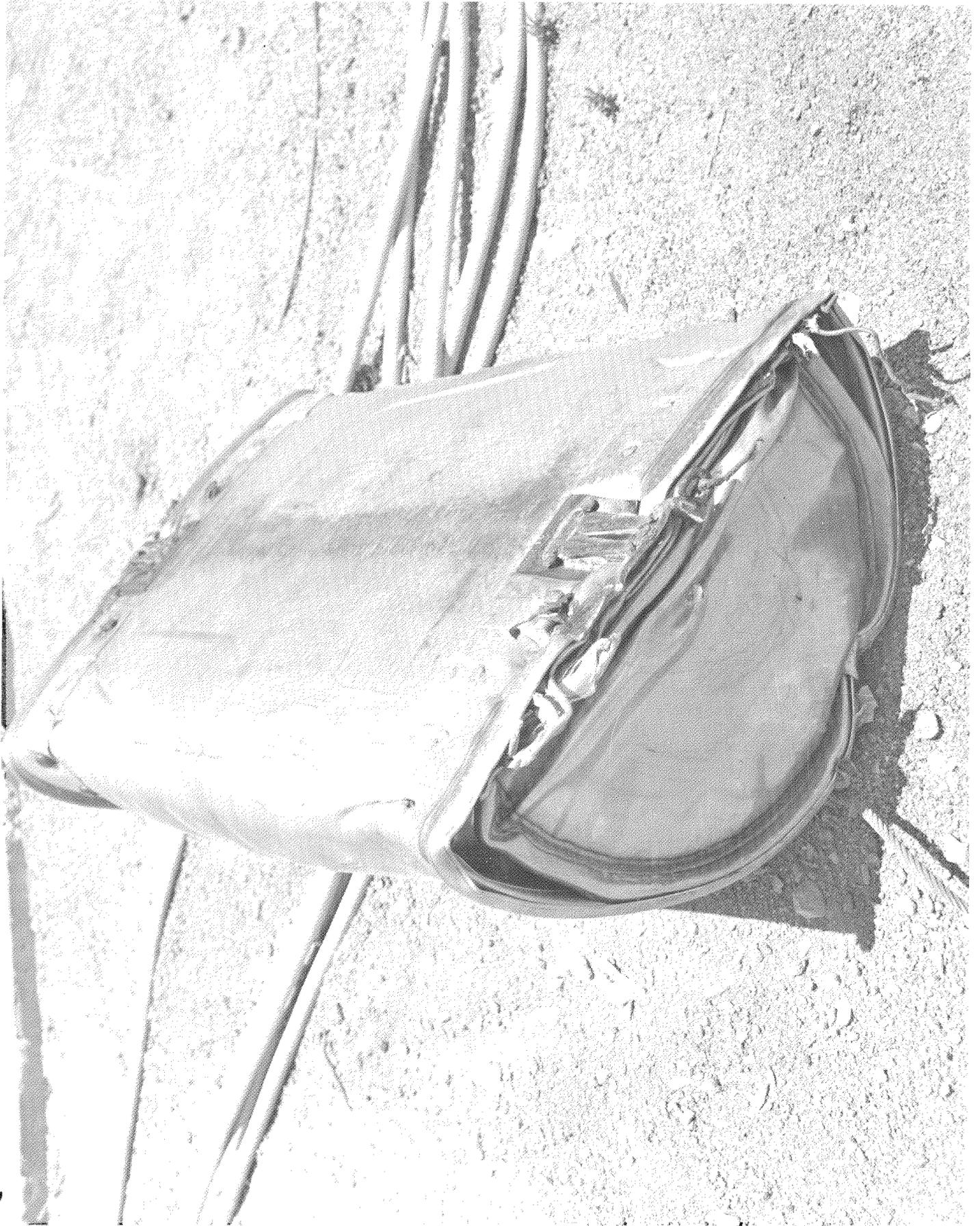
**Fig. 5. PAT-1 Package After Pull-down Test**
