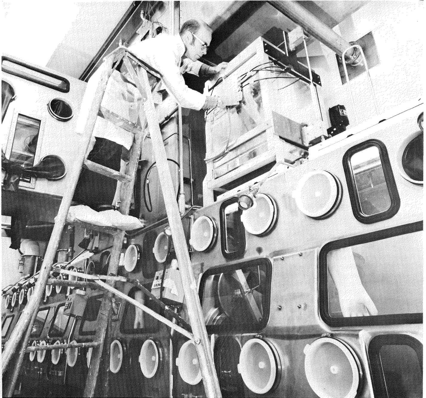
**Bob Marshall, Q-3, focuses attention to a thermal neutron coincidence counter on a glovebox in an area of the facility where fuel pellets are made. Any container of nuclear material that is to be transferred out of this work area must be subjected to monitoring of the neutron counter.**
