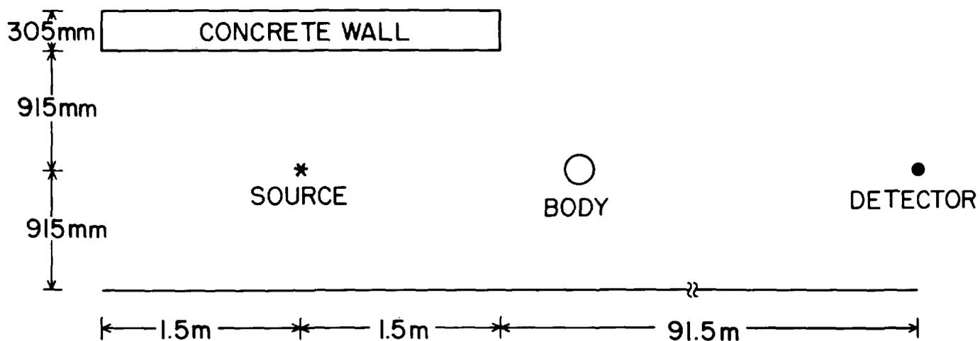
Figure 1. Top view of the model used in the Monte Carlo gamma-ray transport calculations.
