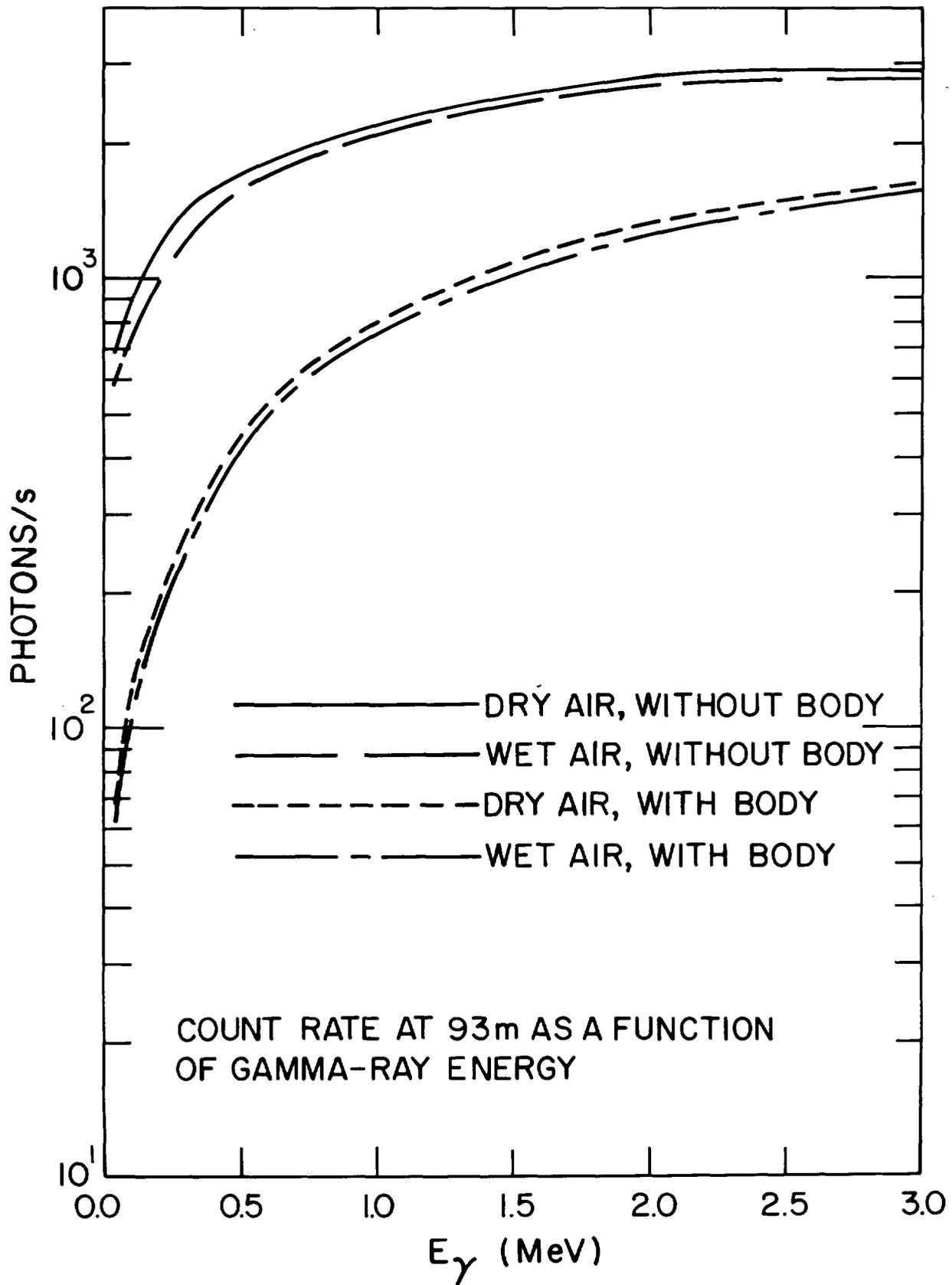
Figure 2. Expected count rates for a source-detector distance of 93 m as a function of the gamma-ray energy, for dry and wet air, and with and without a body in the beam. These curves assume a 1-Ci source and a 100% efficient 127-by 127-mm NaI detector.
