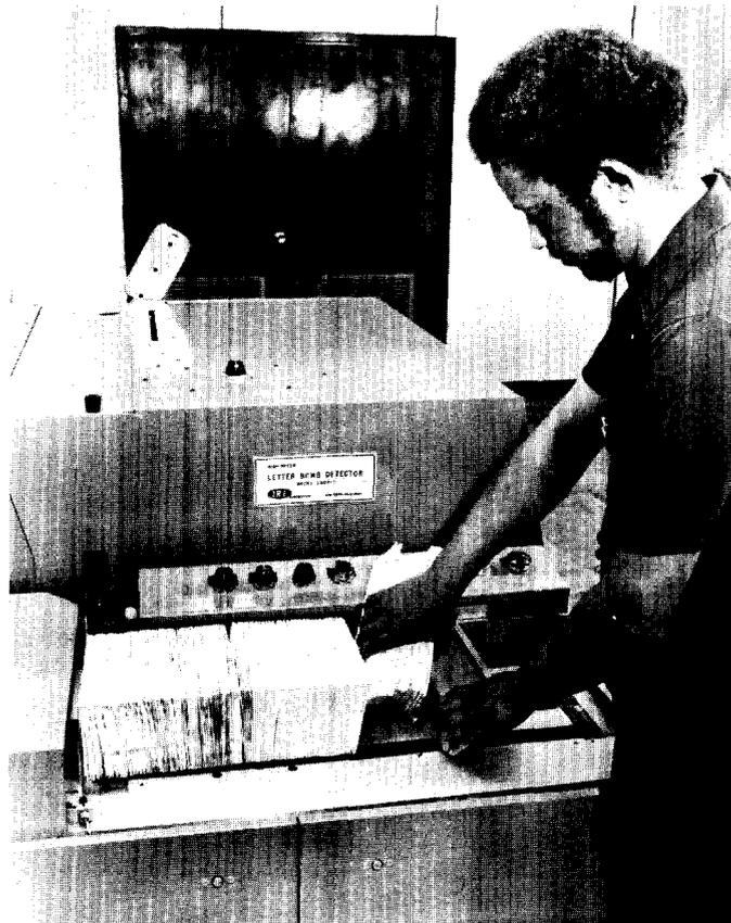
**High speed letterbomb detector, developed by IRT Corporation of San Diego, processes test run of mail as R.J. Michaels, IRT engineer, feeds stacks of sample letters to the system. The detector has been delivered to Washington, D.C., to serve a federal agency.**
