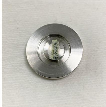
Figure 2. SUDA sampler consisting of a cylindrical aluminum foam loaded with zeolite and mounted on a standard KF-16 fitting.
