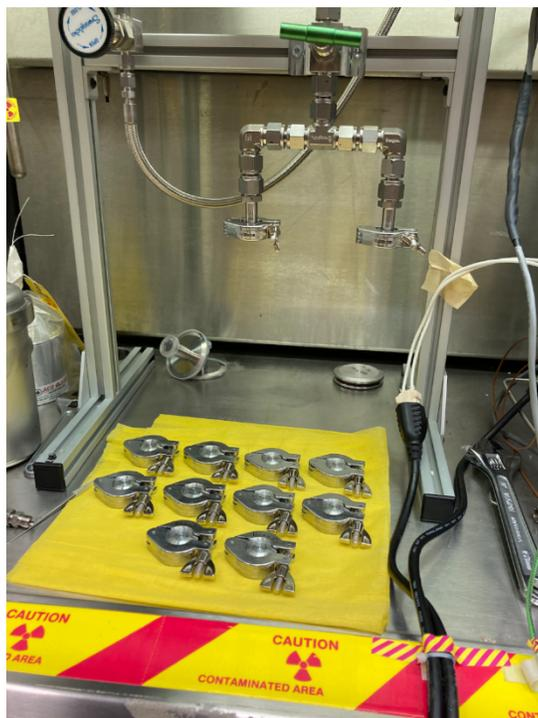
Figure 62. A set of SUDA samplers used to collect  $UF_6$ .
